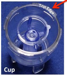
To assemble the VixOne properly, squarely align the cap with the cup and press down lightly to fit them together. Rotate slightly to engage the Tabs underneath the bayonet Slides. Then, rotate clockwise to ride down the Slope and across the Flat until slight resistance is felt when the Tab hits the Stop. The cap is now properly installed on the cup. DO NOT OVER-TIGHTEN. DOING SO WILL STRIP THE END STOP AND PREVENT A LEAK-PROOF SEAL.
